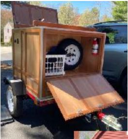
The radio compartment at the rear of the trailer has an access panel that lifts up and is supported by chains that anchor to the top of the box. Inside are radios that are
