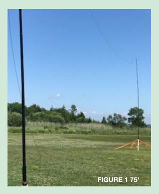
The feedline (RG-8X) length was chosen so as not to be harmonically related to any of the bands being covered. During the construction phase, I was in contact with KC1HQB Ray Vilnit, K1ETA Mike Kenney and K1WMC Mickey Callahan.. Their suggestions facilitated construction of the PVC push up pole supports. Mike had already completed a support system and his input made my assembly go quickly without many retries.
